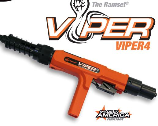
The new Ramset® **VIPER4** .27 Caliber Strip Powder Tool design makes overhead applications even easier. The load advance is now located internally to allow a push/ sleeve actuated operation. *Compatible with the newly designed poles*, the rear collar is connected by set-screw to avoid a manual tightness check.
